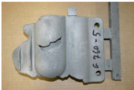
(a) N5181-5c, no vacuum, not filled, misrun.
