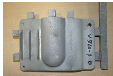
(b) N5181-1c, vacuum, (-40kPa), filled.
