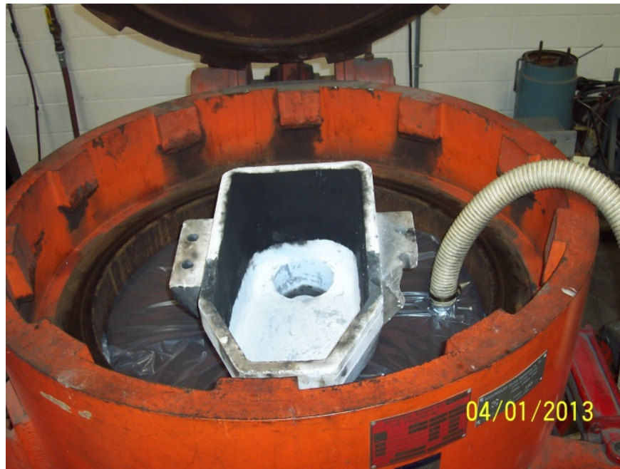
Figure 4.4.6 Flask showing pouring basin inside pressure vessel.
