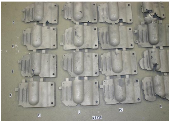
(a) N5230, AZ91D Castings poured at 725°C (127°C superheat).
