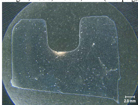
Figure 4.4.13 Porosity of Casting C, A356, 1450°F, VAP (0 psig) and SUP (150 psig), Bearing #4.
