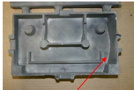
Compaction defect (b) N5181-3c, front.
