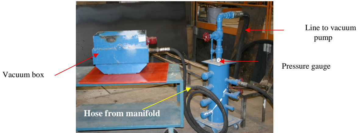
Figure 4.2.1 Vacuum box and pressure manifold system.
