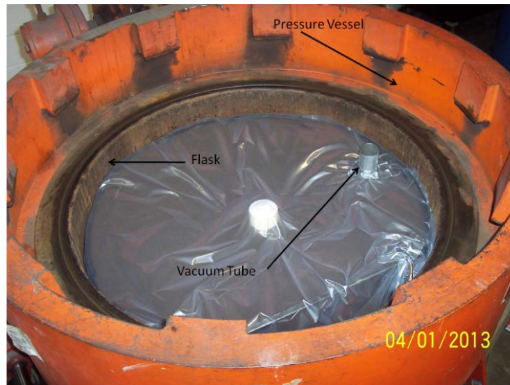
Figure 4.4.4 Experimental flask and vacuum tube inside pressure vessel.
