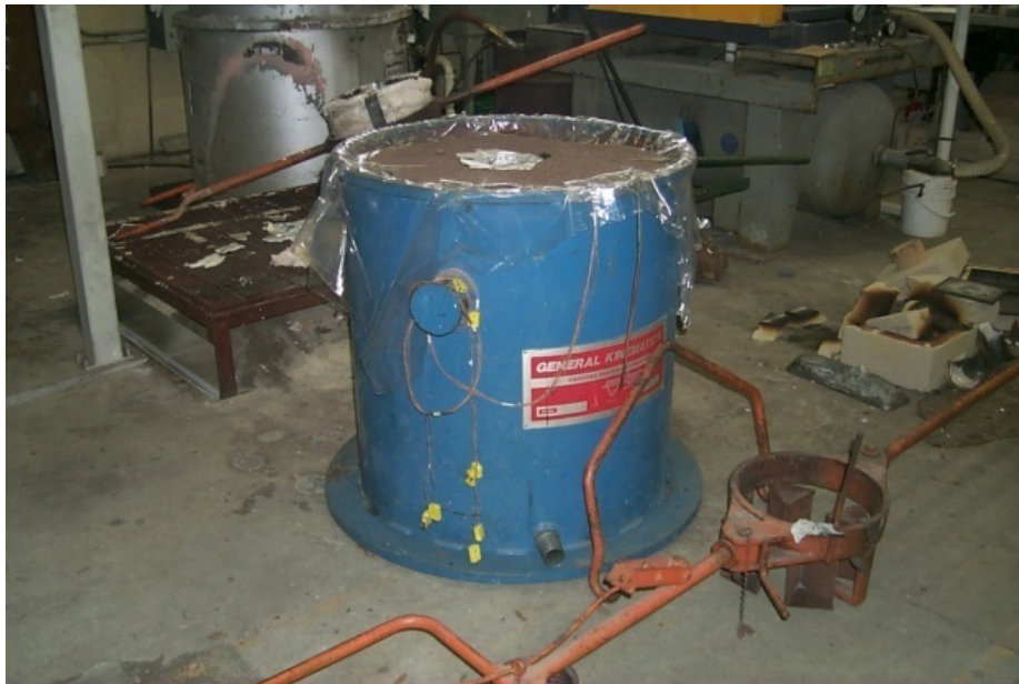
Figure 4.4.3 Molding flask, thermocouples, and pressure instrumentation after pouring.
